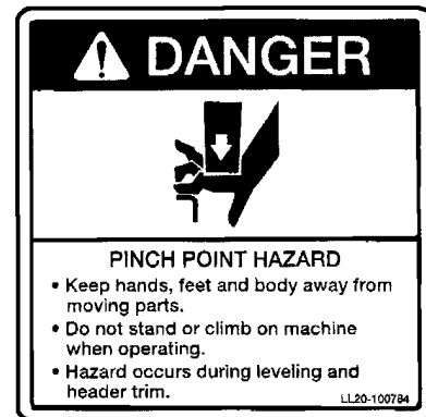
Label #3 Part number: LL20-10784 Locations: 2 (left and right side of upper transition face plate)
