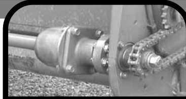
Right Side - Slip Clutch with shield removed
