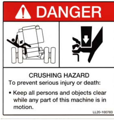
Label #2 Part Number: LL20-100783 Locations: 6 (Front of undercarriage and above rear axle)
