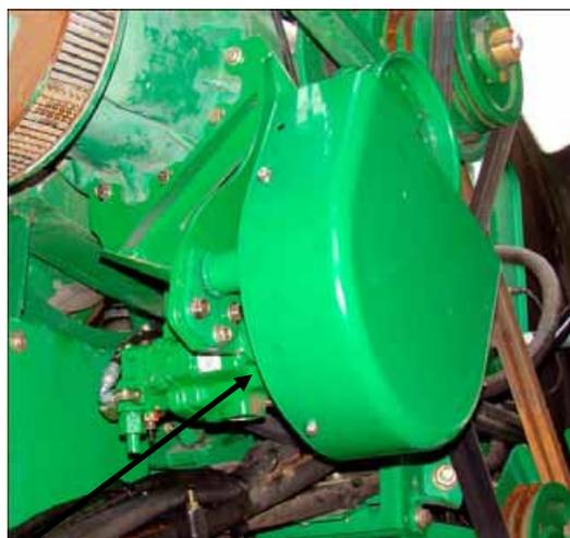
Overhung Load Adapter filled with 2.5 fl. oz. of SHC 526 Synthetic Hydraulic Oil (ISO 68)
