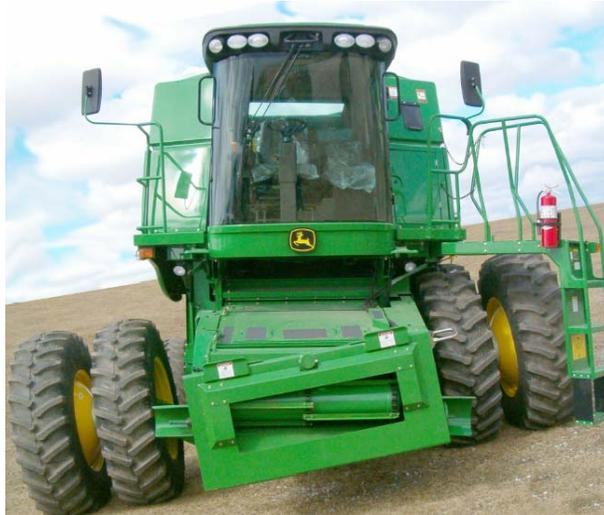
The Hillco Sidehill Leveling system designed for John Deere STS combines. Hillco designed to maintain the STS combine's thrashing capacity and efficiency on contours of up to slopes of 18%. We designed this leveling system to be installed with little modification to the combine.
