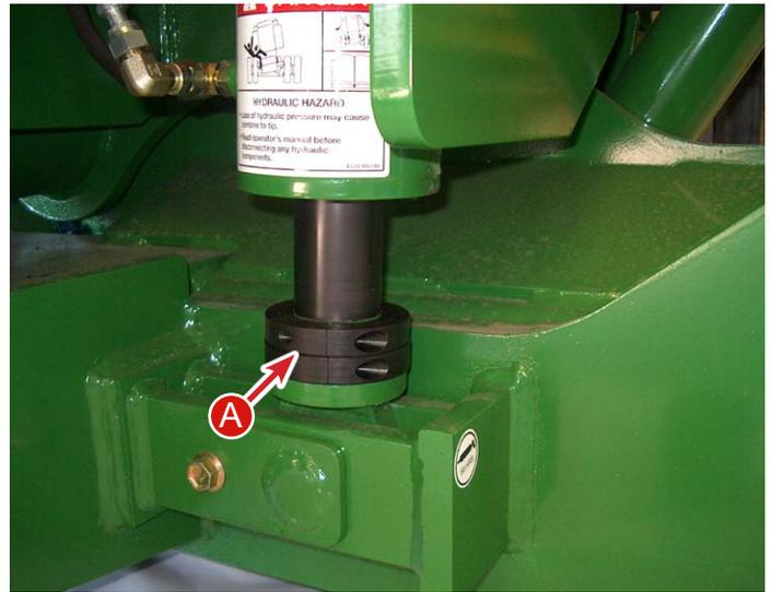
A - Mechanical Leveling Cylinder Stops
