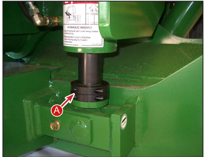
A - Mechanical Leveling Cylinder Stops
