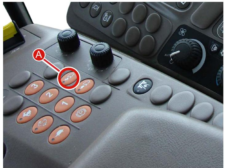
If the combine is not equipped with 4WD the 4WD drive buttons must be deactivated. Follow the steps to activate the 4WD and set the numbering sequence from XXXXXX1X to XXXXXX0X.
