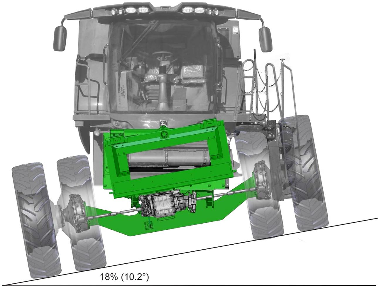
The Hillco Sidehill Leveling System is designed for John Deere S Series combines. Hillco designed the Sidehill Leveling System to maintain the combine's thrashing capacity and harvesting efficiency on contours of slopes up to 18%. This leveling system is designed to be installed with little modification to the combine.
