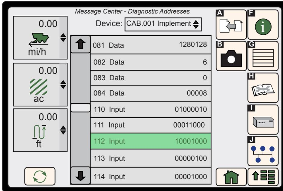
Select the XXXXXXnX numbering sequence by pressing the
