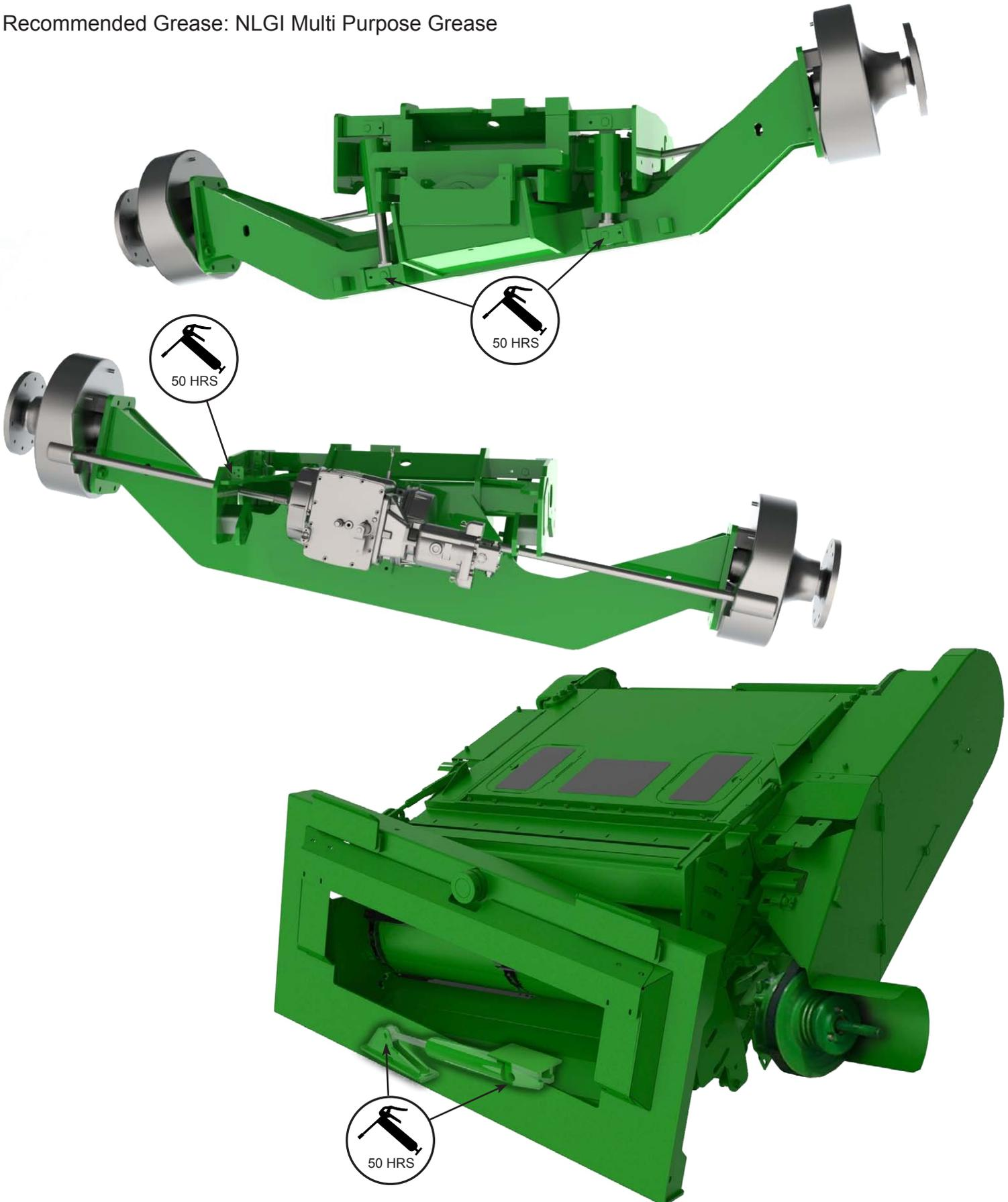
The Transition Pivot Pin and the Rear Drop Axle Spacer utilize Graphite Micarta Bushings that do not require grease.
