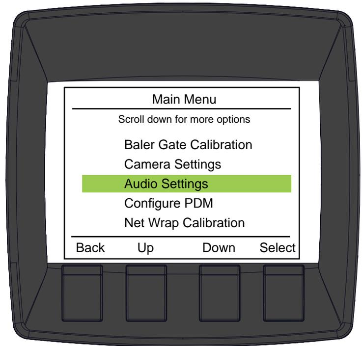
Use the UP (A) and DOWN (B) buttons to toggle between settings. When the desired setting is highlighted press the ENTER (C) button to toggle ON or OFF.
