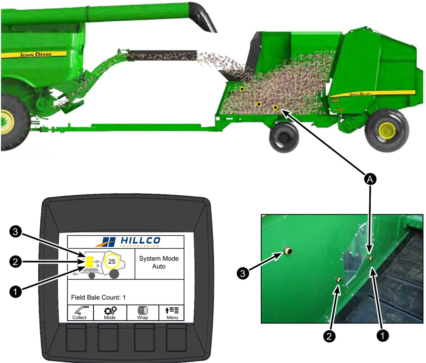
Material is fed from the Accumulator into the baler by the conveyor(A). The feed rolls (B) rotate in the opposite direction of the conveyor, creating a rolling action. This allows for even feeding of the material into the baler. When the Accumulator's fill level is below the bottom infrared light sensor, the feed system and baler disengage and the Accumulator begins to collect material. This process is repeated until the bale reaches the desired size.
