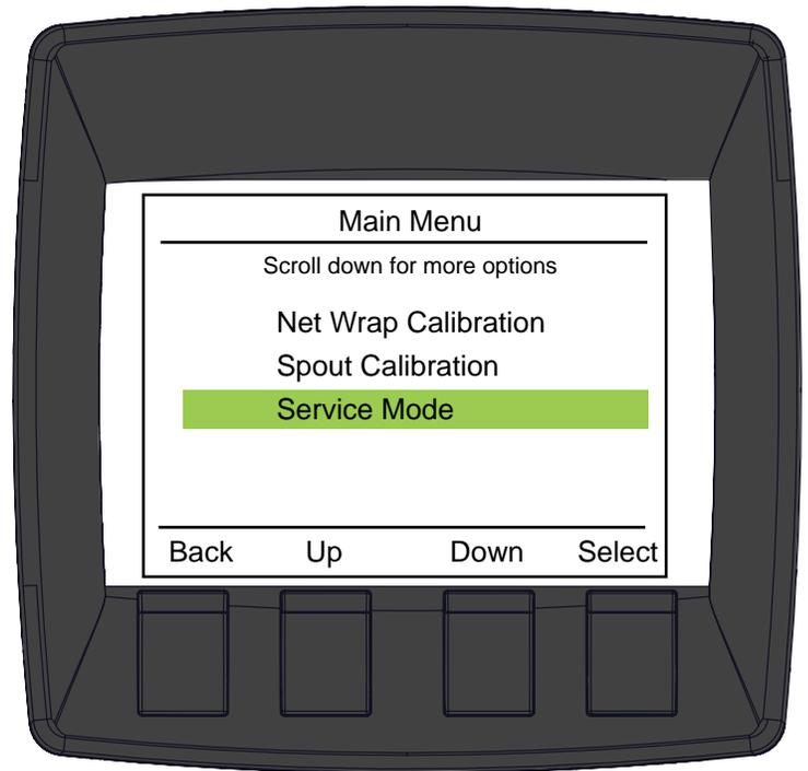
Service Mode allows for manual control of the baler gate, accumulator feed system and baler drive. The screen shows the current RPM's.
