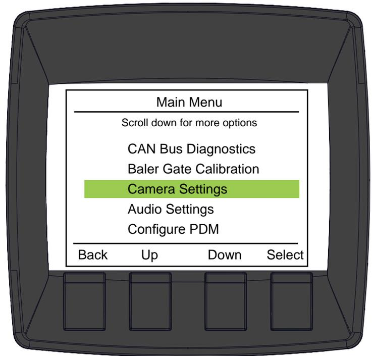
Use the UP (A) and DOWN (B) buttons to toggle between settings. When the desired setting is highlighted press the ENTER (C) button to toggle ON or OFF or to increase the amount of seconds for the Bale View Timer.
