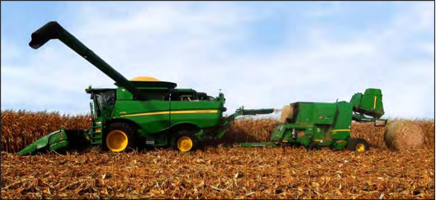
The Hillco Single Pass Round Bale System is designed for John Deere S-Series S670, S680 & S690 ProDrive Combines and 569 Standard Round Balers. Hillco designed the SPRB System to allow for continuous round baling of crop residue known as Material Other than Grain (MOG).
