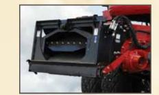
The CH7010 and CH9010 utilize a low maintenance paddle beater feed system to allow for extra header rotation and is designed for maximum throughput to handle the heaviest of yields.
