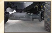
**REAR DROP AXLE**—The drop axle lifts the rear of the combine to match the height increase of the overcarriage/undercarriage. This levels the combine fore/aft and accommodates both powered and non-powered rear axles.
