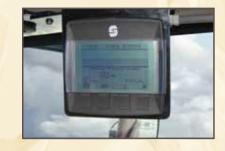
**MONITOR**—An in-cab monitor is used to display warnings and to provide electrical diagnostic information.
