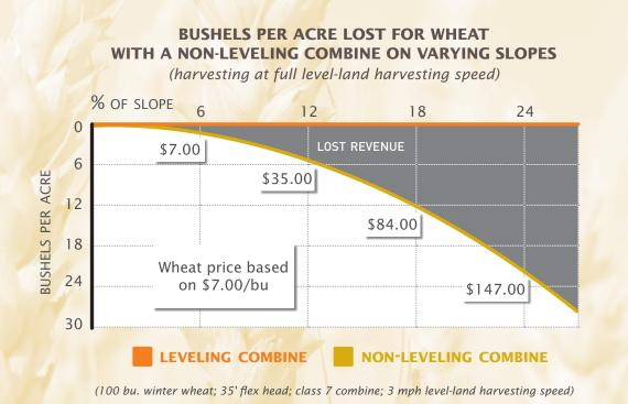
As a non-leveling combine moves onto a hillside, threshed material moves to the low side of the cleaning shoe, allowing valuable cleaning air to escape without lifting and separating the crop. The result is hillside grain loss.
