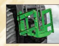
**LADDER**—A retractable double step ladder is installed to the bottom of the John Deere ladder, allowing for easier access to the cab.
