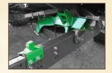
**REAR DROP AXLE**—The drop axle lifts the rear of the combine to match the 8" height increase of the overcarriage/undercarriage. This levels the combine fore/aft and accommodates both powered and non-powered rear axles.
