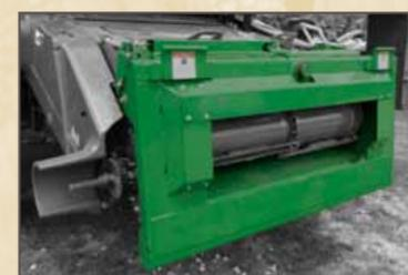
**CROP FEEDING SYSTEM**—The Sidehill header transition extends the feeder chain and provides feeding in all crops and conditions.
