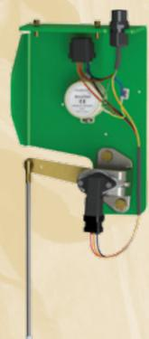
**ADVANCED SLOPE SENSING & CORRECTION**—The clinometer-based slope sensor mounted to the carriage continuously monitors the slope and maintains a level combine chassis. The technology utilized in the leveling controller and hydraulic control valve allows for variable leveling speed.
