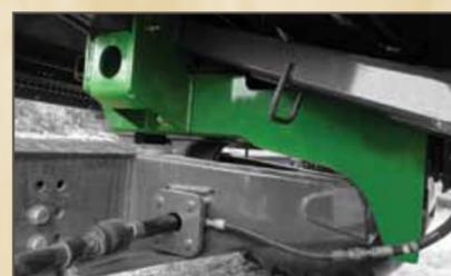
**REAR DROP AXLE**—The drop axle lifts the rear of the combine to match the 7" height increase of the overcarriage/undercarriage. This levels the combine fore/aft and accommodates both powered and non-powered rear axles.
