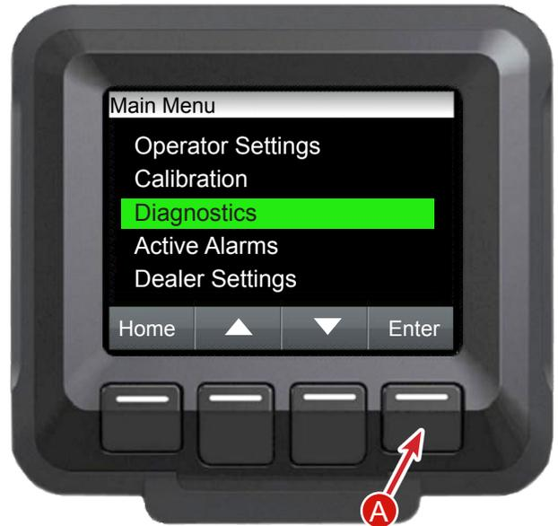
The Diagnostics menu allows the operator to view output information from the electrical system on the leveling system.
