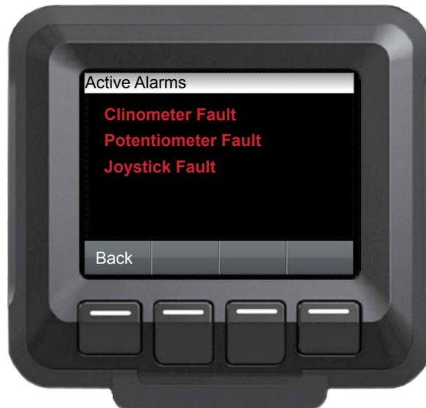
Potentiometer Fault (Carriage Angle Sensor Fault)
