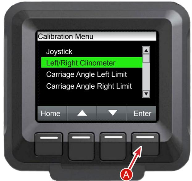
Follow the directions on the screen. When the combine is level side to side press Enter (A).
