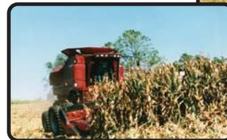
**Maximum Hillside Capacity** - The Model 2800's 27% slope compensation is complemented by the hillside efficiency of the rotary combine, giving you a hillside combine built to deliver optimum cleaning performance and capacity in the world's steepest terrain. The front drive tires are moved forward to improve fore-aft balance for better downhill performance.
