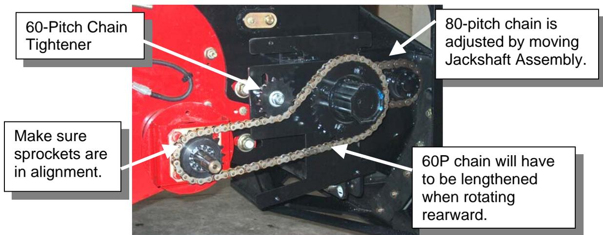
Do not over tighten these sprockets or premature chain and sprocket wear will occur.
