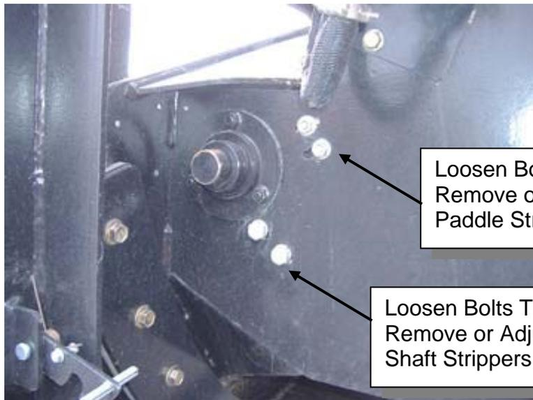
Loosen Bolts To Remove or Adjust Paddle Strippers
