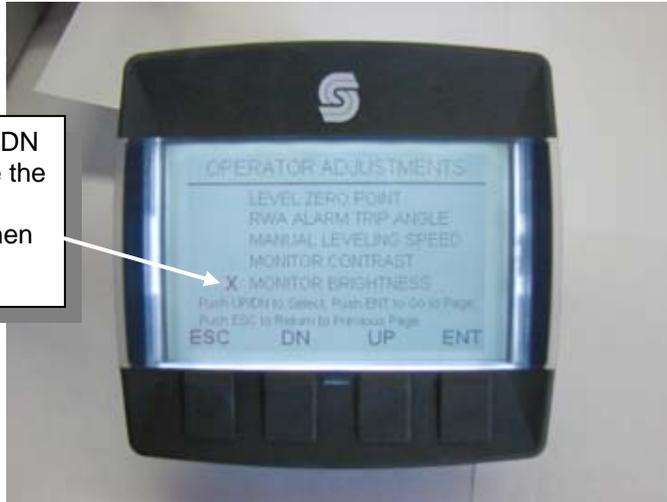
Once in the Manual Leveling Speed Screen, push the **UP** or **DN** buttons to increase or decrease the manual leveling speed (Default Setting is 13). Once the desired setting is reached on the bar graph, push and hold the **ENT** button for 1 second. This will lock the new manual leveling speed setting. When done push the **ESC** button to leave the page. Note: Pushing the **ESC** button will take you back to the Menu Screen.
