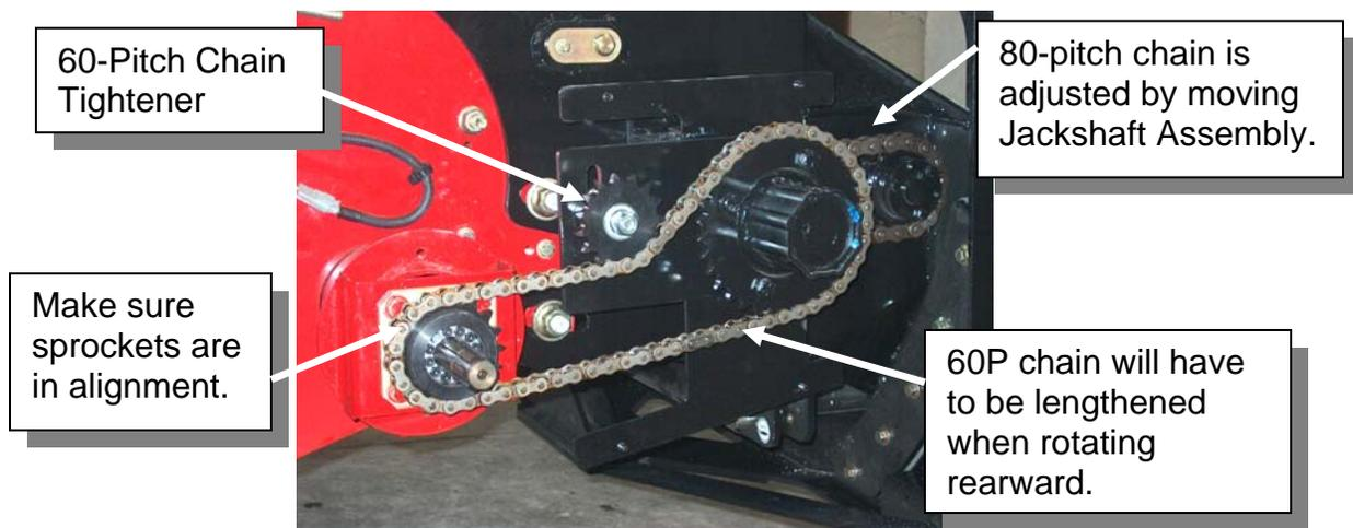
Do not over tighten idler sprockets or premature chain and sprocket wear will occur.
