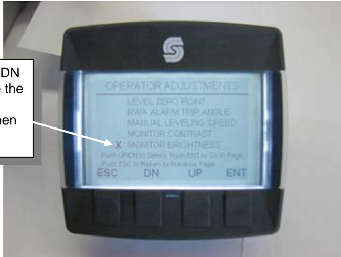
Once in the Monitor Contrast Screen, push the **UP** or **DN** buttons to increase or decrease the contrast (Default Setting is -3). Once the desired setting is reached, push and hold the **ENT** button for 1 second. This will lock the new monitor contrast setting. When done push the **ESC** button to leave the page. Note: Pushing the **ESC** button will take you back to the Menu Screen.
