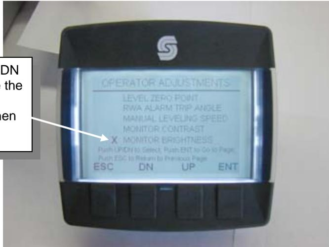
Once in the Monitor Brightness Screen, push the **UP** or **DN** buttons to increase or decrease the brightness (Default Setting is 8). Once the desired setting is reached, push and hold the **ENT** button for 1 second. This will lock the new monitor brightness setting. When done push the **ESC** button to leave the page. Note: Pushing the **ESC** button will take you back to the Menu Screen.
