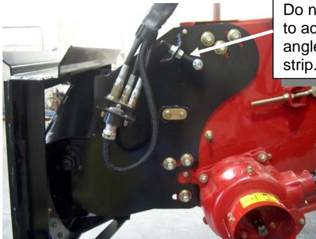
Do not use the eyebolt to adjust the header angle. The threads will strip.
