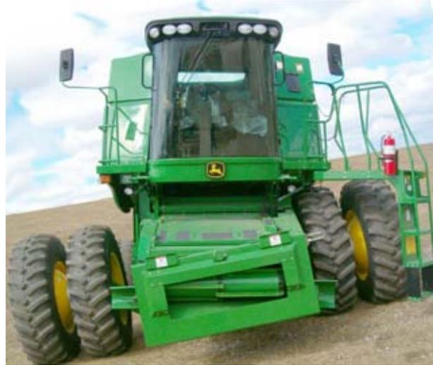
The leveling system uses a clinometer to sense the combine chassis position relative to level. As the combine moves onto a slope, the chassis leans out of level, the clinometer senses the deviation and sends a signal the controller. The controller opens the appropriate leveling valve. The leveling valve allows hydraulic oil to flow into the leveling cylinder. The cylinders tilt the combine chassis to correct for the chassis tilt, bringing the chassis back to level.
