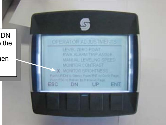
Once in the Level Zero Point Screen place a level on the cab floor. Manually level the combine to the left (**L**) or right (**R**) until the bubble shows level. Push and hold the **ENT** button for 1 second. This will set the Zero Point for Leveling. This is a one (1) time adjustment unless the clinometer or controller has been replaced. When done push the **ESC** button to leave the page. Note: Pushing the **ESC** button will take you back to the Menu Screen.
