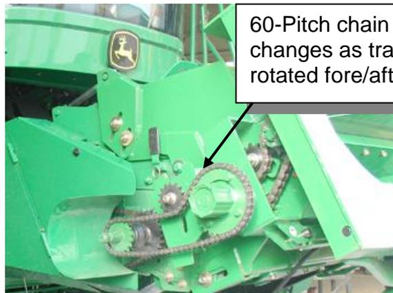
60-Pitch chain length changes as transition is rotated fore/aft.
