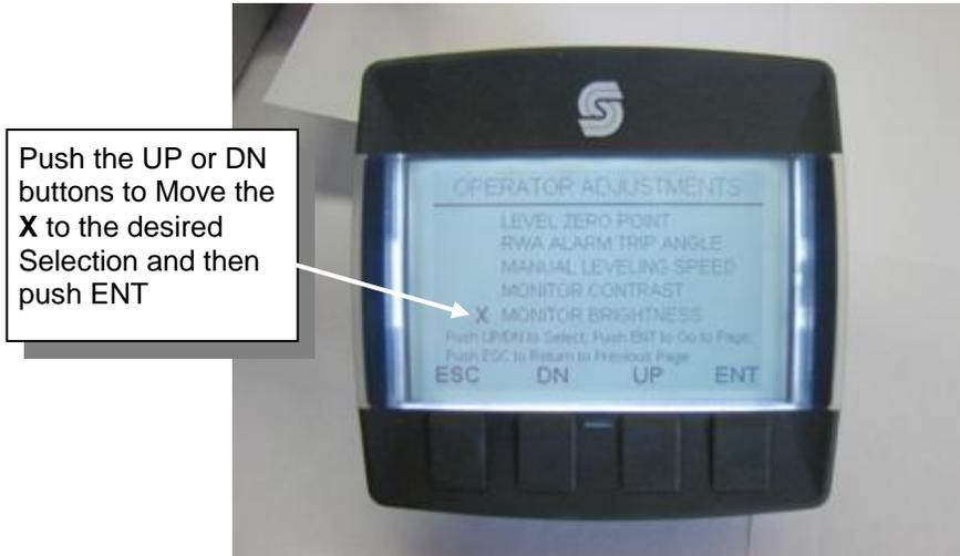
Once in the Monitor Contrast Screen, push the **UP** or **DN** buttons to increase or decrease the contrast (Default Setting is -3). Once the desired setting is reached, push and hold the **ENT** button for 1 second. This will lock the new monitor contrast setting. When done push the **ESC** button to leave the page. Note: Pushing the **ESC** button will take you back to the Menu Screen.
