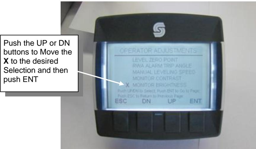
Once in the Manual Leveling Speed Screen, push the **UP** or **DN** buttons to increase or decrease the manual leveling speed (Default Setting is 13). Once the desired setting is reached on the bar graph, push and hold the **ENT** button for 1 second. This will lock the new manual leveling speed setting. When done push the **ESC** button to leave the page. Note: Pushing the **ESC** button will take you back to the Menu Screen.
