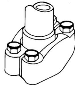
***DO NOT USE AIR WRENCHES. DO NOT TIGHTEN ONE CAP SCREW FULLY BEFORE TIGHTENING THE OTHERS. DO NOT OVER TIGHTEN.***
