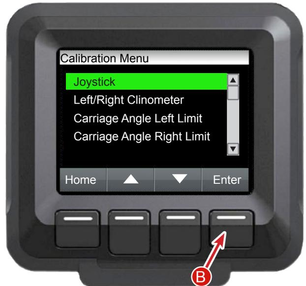
With the Joystick in the center position press the Enter button (C).
