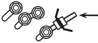
Do Not use Eyebolt to Adjust Header Angle or Threads will Strip.
