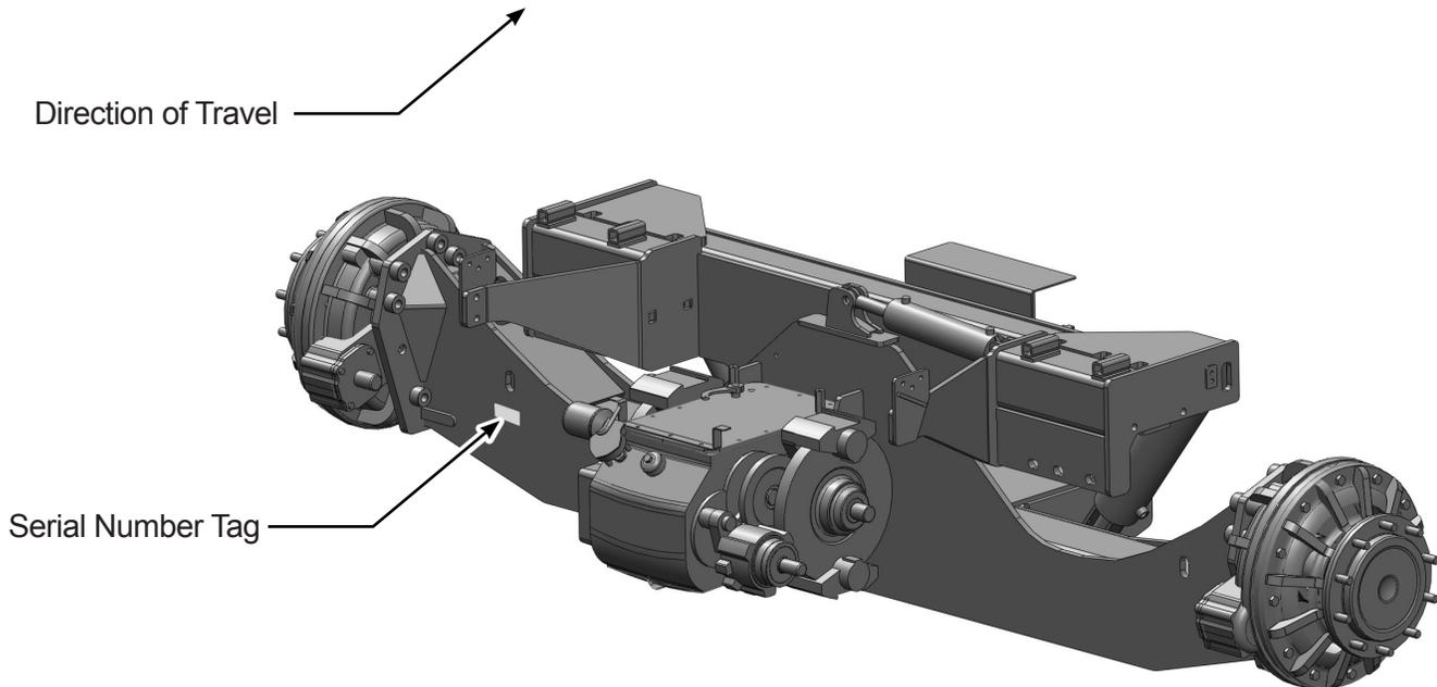
Write the serial number and the model number of the leveling system and combine on the lines provided. It is important to reference these numbers when ordering parts or requesting technical support. We suggest that you give the leveling system serial number to your Case IH dealer to be kept with their combine serial number records.
