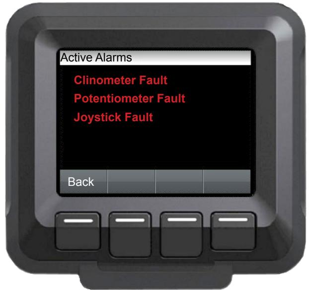
Potentiometer Fault (Carriage Angle Sensor Fault)
