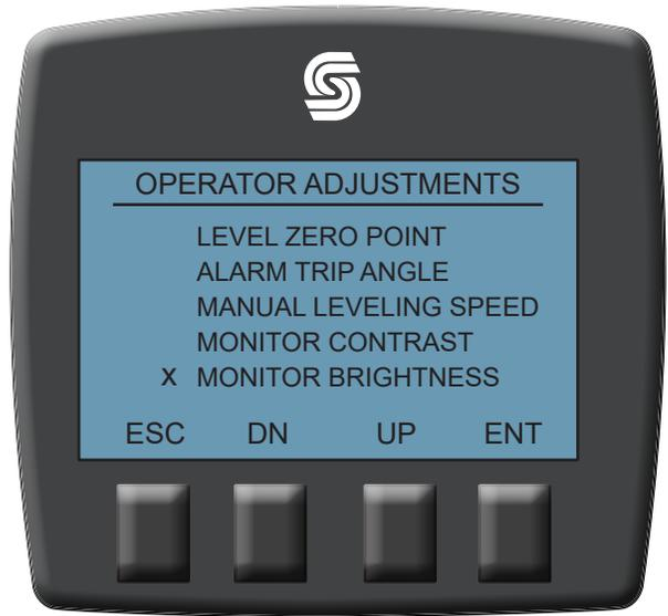
Once in the Monitor Brightness Screen, push the UP or DN buttons to increase or decrease the brightness (Default Setting is 8). Once the desired setting is reached, push and hold the ENT button for 1 second. This will lock the new monitor brightness setting. When done push the ESC button to leave the page.
