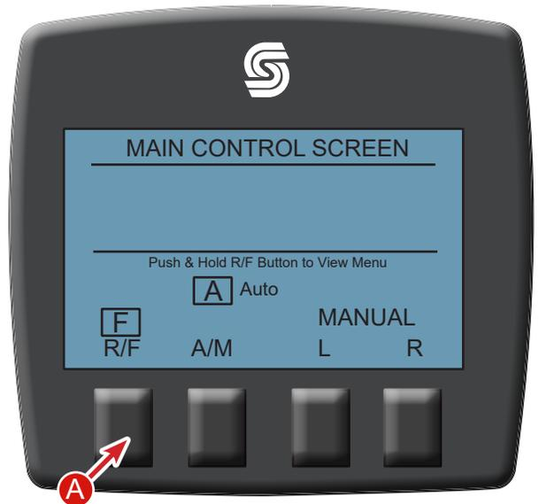
Push the UP (C) or DN (B) buttons to move the X to the Operator Adjustments Line and then push the ENT (D) button to go into that Page. Note: Pushing the ESC (A) button will take you back to the Main Control Screen.
