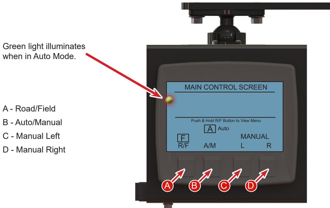
**Remote Leveling Switches:** Located to the right of the armrest control panel. These switches allow for Auto/Manual control and Left/Right leveling.
