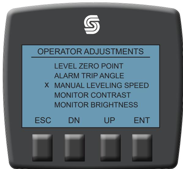
Once in the Manual Leveling Speed Screen, push the UP or DN buttons to increase or decrease the manual leveling speed (Default Setting is 13). Once the desired setting is reached on the bar graph, push and hold the ENT button for 1 second. This will lock the new manual leveling speed setting. When done push the ESC button to leave the page.
