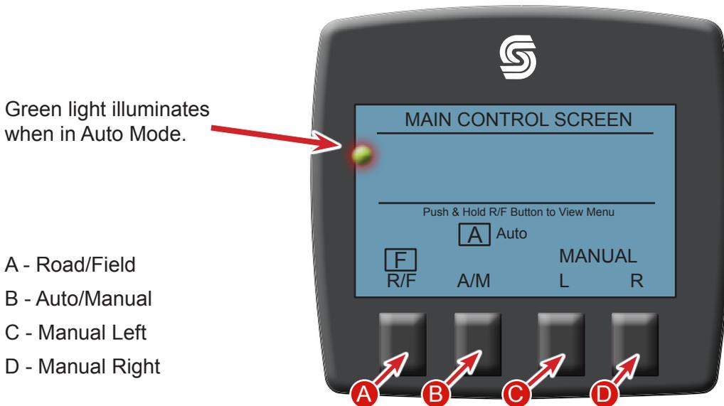
**Remote Leveling Switches:** Located on the armrest control panel. These switches allow for Auto/Manual control and Left/Right leveling.
