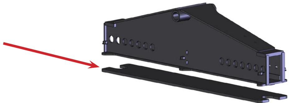
Use caution when using individual turning brakes. Installation of a Hillco Leveling System transmits additional weight to the rear axle of the combine. Excessive braking to turn can damage your combine chassis.
