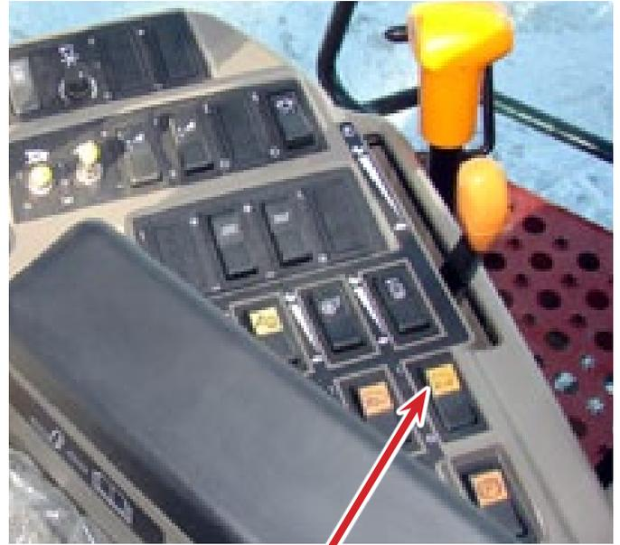
Rear Wheel Assist Engage/Disengage
