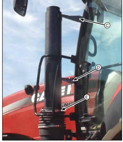
Install the pre-cleaner to the intake tube. Press the intake all the way down onto the tube. Make sure that the slits in the pre-cleaner are covered so that all air entering has to go through the pre-cleaner.
