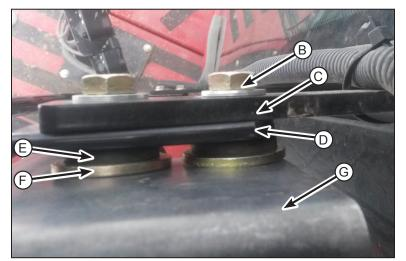
Secure the intake mounts with the original washers and nuts. Tighten to prevailing torque.
