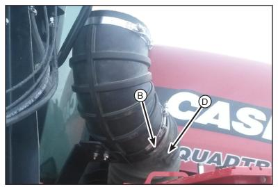
Do not tighten the original clamp (D) because the elbow may need to be rotated when installing the intake tube.
