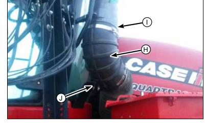
Install the pre-cleaner to the intake tube. Press the intake all the way down onto the tube. Make sure that the slits in the pre-cleaner are covered so that all air entering has to go through the pre-cleaner.
