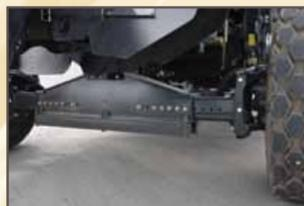
**REAR DROP AXLE**—The drop axle lifts the rear of the combine to match the height increase of the overcarriage/undercarriage. This levels the combine fore/aft and accommodates both powered and non-powered rear axles.
