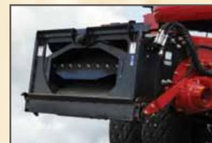
The CH7010 and CH9010 utilize a low maintenance paddle beater feed system to allow for extra header rotation and is designed for maximum throughput to handle the heaviest of yields.
