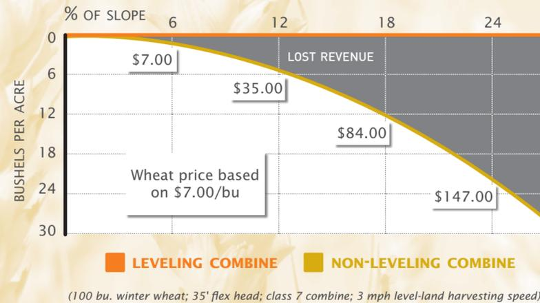
As a non-leveling combine moves onto a hillside, threshed material moves to the low side of the cleaning shoe, allowing valuable cleaning air to escape without lifting and separating the crop. The result is hillside grain loss.
