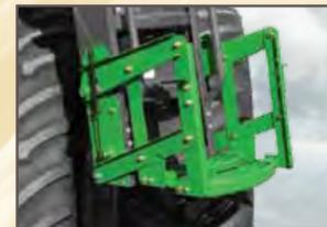
**LADDER**—A retractable double step ladder is installed to the bottom of the John Deere ladder, allowing for easier access to the cab.
