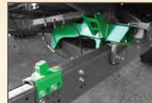
**REAR DROP AXLE**—The drop axle lifts the rear of the combine to match the 8" height increase of the overcarriage/undercarriage. This levels the combine fore/aft and accommodates both powered and non-powered rear axles.
