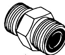
**NOTE: DO NOT ALLOW HOSES TO TWIST WHEN TIGHTENING FITTINGS**
