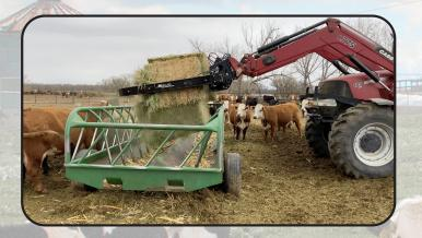
Square bales can be fed into feed pens without the need to get out of the tractor and cut the bale yourself.
