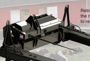
Retractable hooks collect and hold the netwrap or twine until it's ready to realease.
