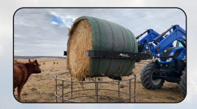
Round bales can be dropped into feed pens without the need to get out of the tractor and cut the bale yourself.
