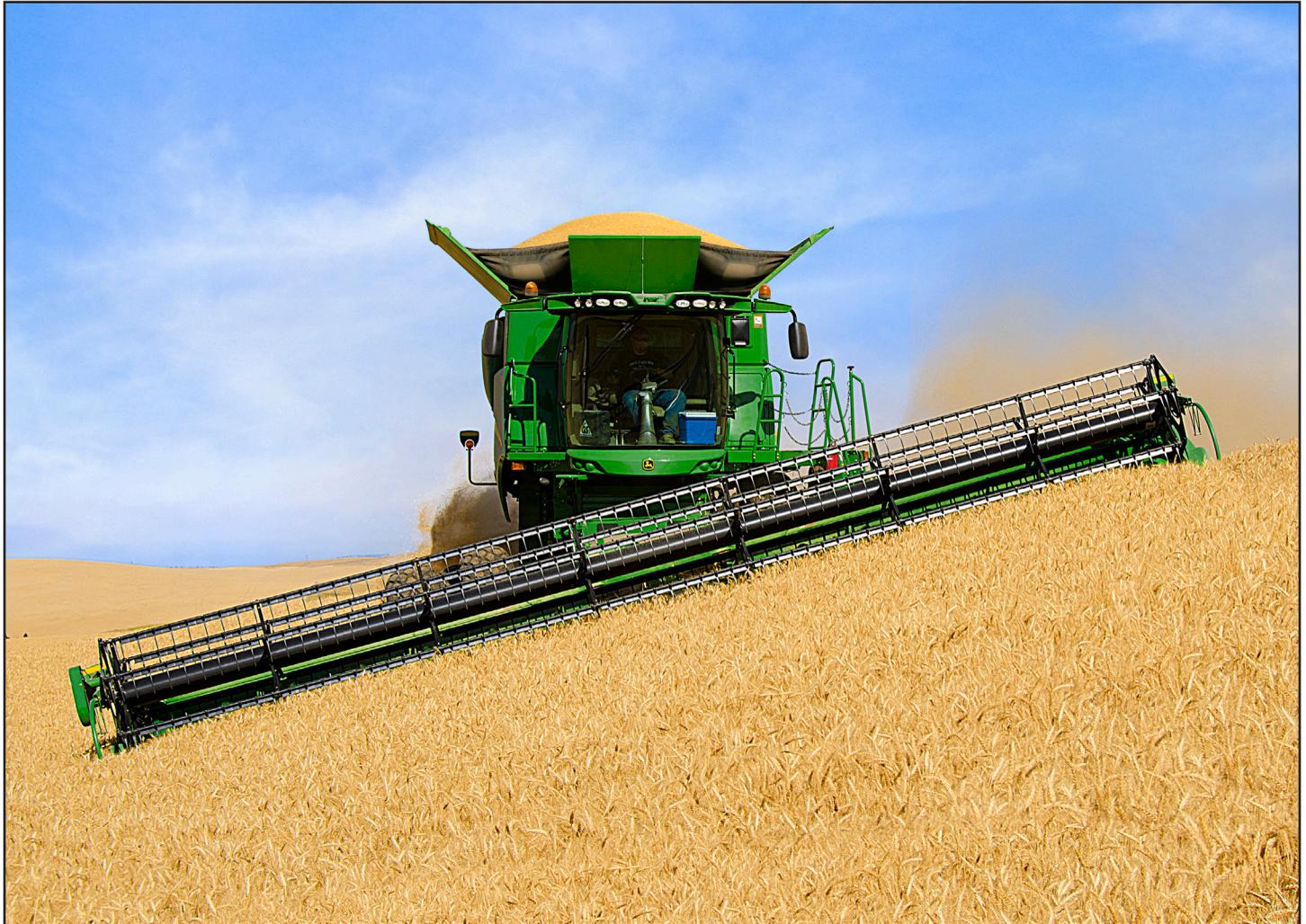
The Hillco Hillside Leveling System is designed for John Deere S Series combines. Hillco designed the Hillside Leveling System to maintain the combine's thrashing capacity and harvesting efficiency on contours of slopes up to 27%. This leveling system is designed to be installed with little modification to the combine.
