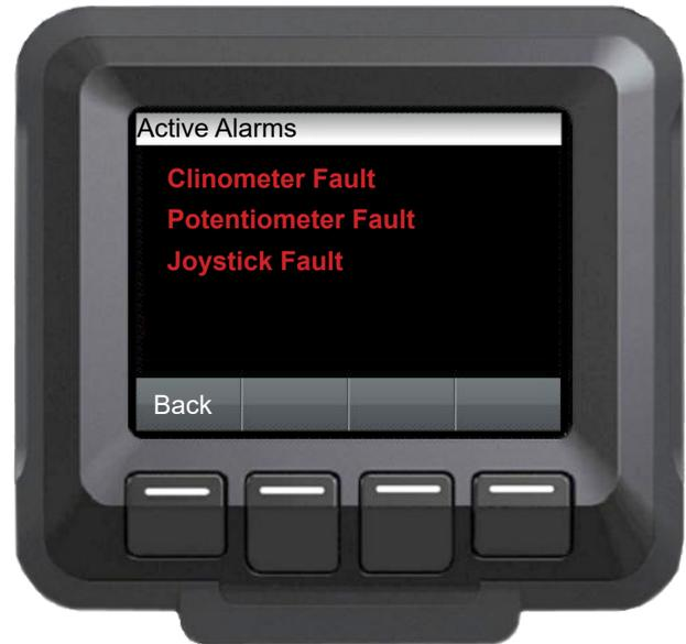
Potentiometer Fault (Carriage Angle Sensor Fault)
