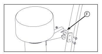
The bottom mount (D) will use 1 M12 x 25 bolt and nut. Install rubber pad between bottom intake mount and cab bracket. The M12 bolt will fit tight into the rubber pad. Leave the mounting bolts loose for now as the intake may need to be shifted around to get the precleaner secured to the top.
