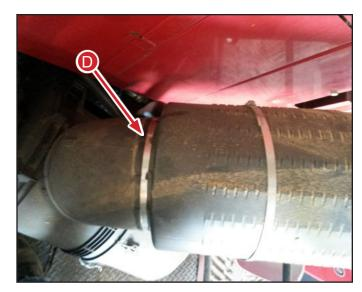
Step 4 - Inspect strata tubes to make sure they are clean. If dirty disasemble from filter housing and clean.
