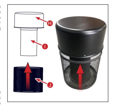
Step 11 - Install precleaner and pipe to rubber elbow.
