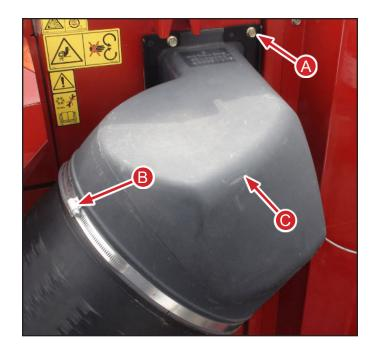
Make sure that the clamp that holds the strato tube onto the bottom elbow is tight. If not when you attempt to remove the elbow it may separate here breaking the silicone seal.
