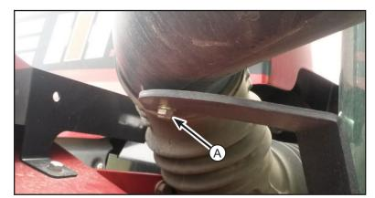
Remove the air intake mounts (C) from the handrail mounts. The mounts may be froze to the isolators. Use a prybar to remove the mount. The isolator and other fasteners will be reused.
