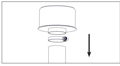
Locate the discharge louver on the side of the pre-cleaner. Rotate the pre-cleaner on the intake tube so that the discharge louver is point to the outside of the tractor.
