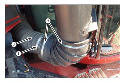
Install the pre-cleaner to the intake tube. Press the intake all the way down onto the tube. Make sure that the slits in the pre-cleaner are covered so that all air entering has to go through the pre-cleaner.
