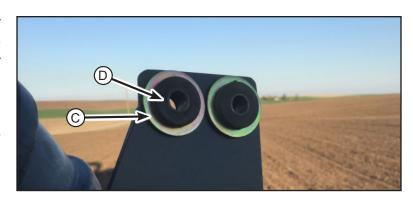
Install the intake tube into the bottom boot. Then align the four mounting holes on the intake tube to the front side of the four handrail mounting bolts as shown. See pictures on the following page.
