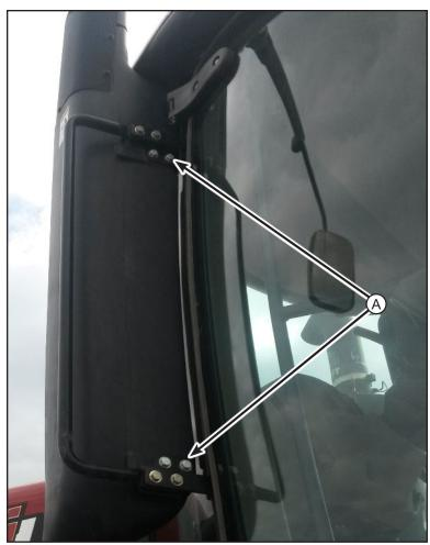
Remove the 3 bolts that secure the bottom of the are intake to the mount.
