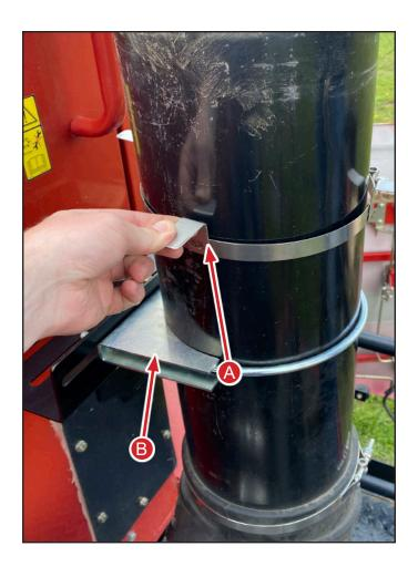
Next, slide the corn screen (C) onto the intake tube so that it rests on top of the support clamp.
