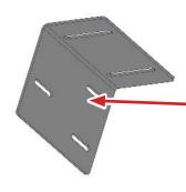
If your combine does not have existing holes for the mount to use then you will need to drill them. Locate the top of the mount roughly 15" above the ring of the 90° elbow. Mark the 3 holes (C) and drill. Verify first there is nothing behind that can be damaged.
