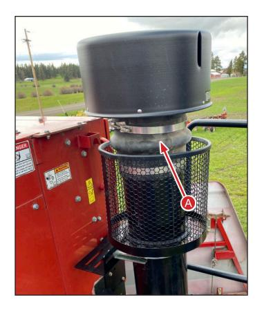
Step 12 – For Kit #CLM7510 only, slide the support clamp and corn screen up until a good seal is made around the base of the Pre-cleaner top. Fasten the support clamp tightly.
