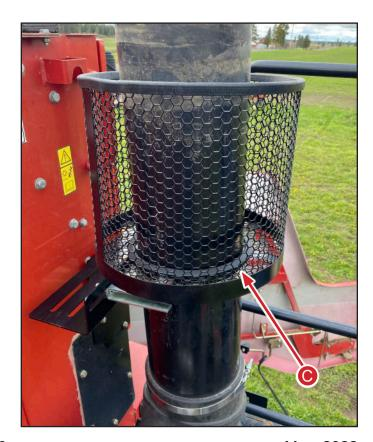
Step 11 – Install the 8" rubber hump hose on top of the intake tube (A). Slide Hump hose on far enough to achieve engagement with the supplied hose clamp. (2 in.) Finally, install the Pre-cleaner top into the hump hose. Verify the Precleaner slides into the hump hose far enough to achieve engagement with the provided hose clamp.
