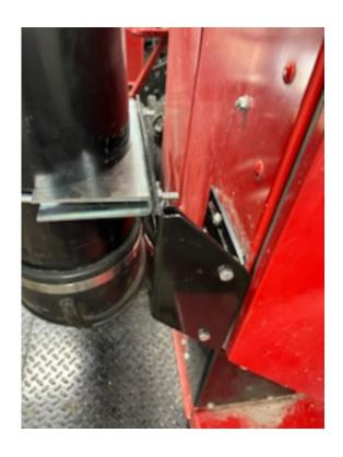
Step 5 - Apply the supplied tile tape to the inside of the coupler (A). This will create a seal between the adapter and the original Case precleaner.
