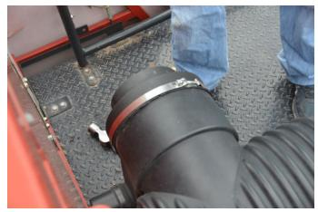
Step 7 - Slide the 8" rubber elbow (A) onto the coupler with the clamps. Insert the 8" tube into the rubber elbow. A spray lubricant may be needed.
