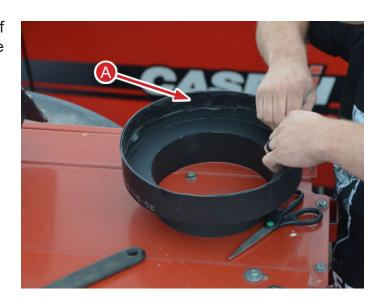
Step 6 - This part of the install can be particularly difficult. Bending the adapter opening slightly to create a bell shape will help. Take care and time to slide the adapter onto the filter housing. This needs to be a tight fit to stop air leaks around the adapter. Once it is in place, use the supplied hose clamp to tighten and seal the adapter.
