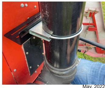
Step 10 - For Kit #CLM7510 only, slide the corn screen support clamp (A) over the intake tube so that it rests on the tube support bracket (B). It will be located at the correct spot later in the installation.
