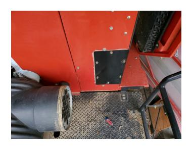
If your 7120 or 8120 is equipped with a wrap around intake, please use the wrap around cover provided.
