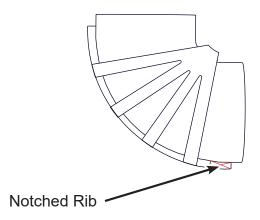
Install the elbow to the tractor. Insert the adapter (B) into the original intake tube (D) and set the elbow on the bottom mount.
