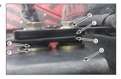
Secure the intake mounts with the original washers and nuts. Tighten to prevailing torque.
