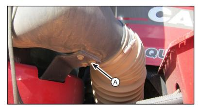
Remove the air intake mounts (C) from the handrail mounts. The mounts may be froze to the isolators. Use a prybar to remove the mount. The isolator and other fasteners will be reused.
