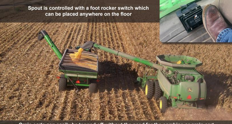
Grain carts can easily be topped off without the need for the combine or grain cart to shift positions relative to each other.
