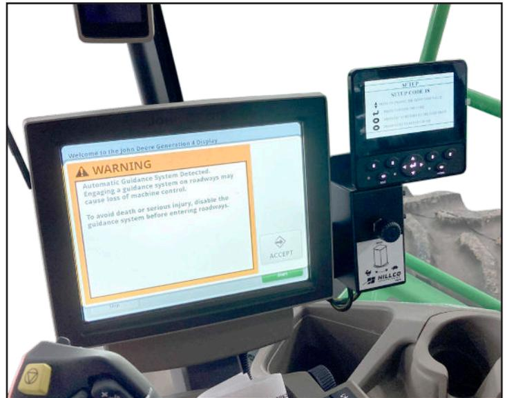
The operators station has a yellow switch to turn on the header and the large control screen 4600 from JD shown here. On the right side of the large screen is the control screen for the Legacy AIR system and the encoder knob.
