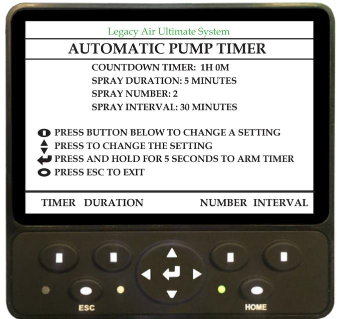
Follow on screen instructions correctly and you will see "Timer Armed". You can turn off the key. The system will wake up and do the spray when commanded.
