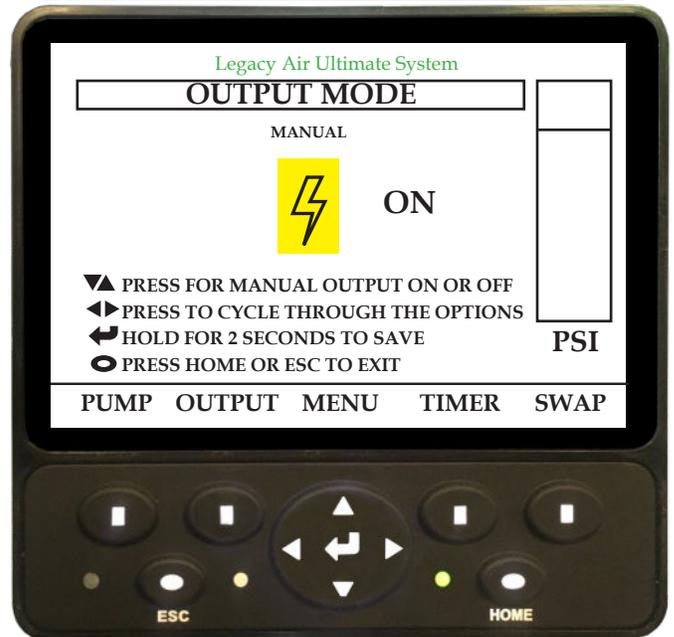
Output mode is for a trigger wire is integrated into the harness that runs back to the solution pump. That trigger wire is available to operate a relay to provide power for different customer functions.
