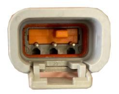
Use a small flat screw driver to release the wire and pin from the connector. Remove the three wires and inspect that the wires are connected to the pins. If they look good reinstall pins in the spots shown above.
