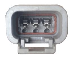
If the three pin connector looks good disassemble the switch box by taking the bottom cover off. Verify the three wires are soldered to the corresponding spades on each switch. If a wire is broke resolder it to the correct spade. The clear wire should be soldered to both switches. The brown and red wire go to the switches as shown.
