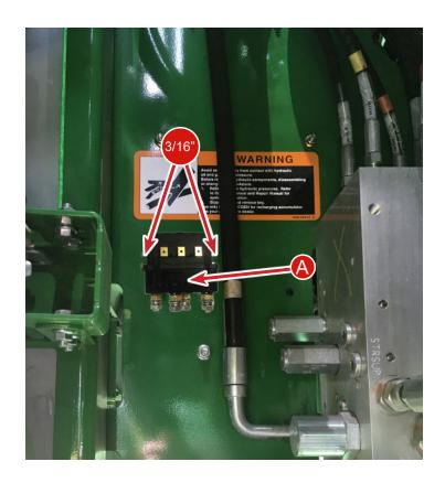
Route harness 1346681 to the actuator control. Cut off excess wire and crimp on ring terminals. The white wire and black wire need to be connected to the two bottom terminals. If after installation is complete the spout pivots the wrong direction these wires can be switched.
