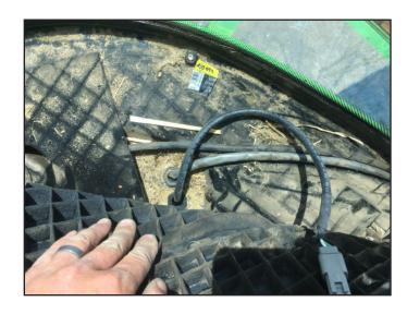
Use a small screw driver to release the clip for each wire (B). Then pull that wire out. When the last wire is released the grey plug will come off. Route harness through strain relief.
